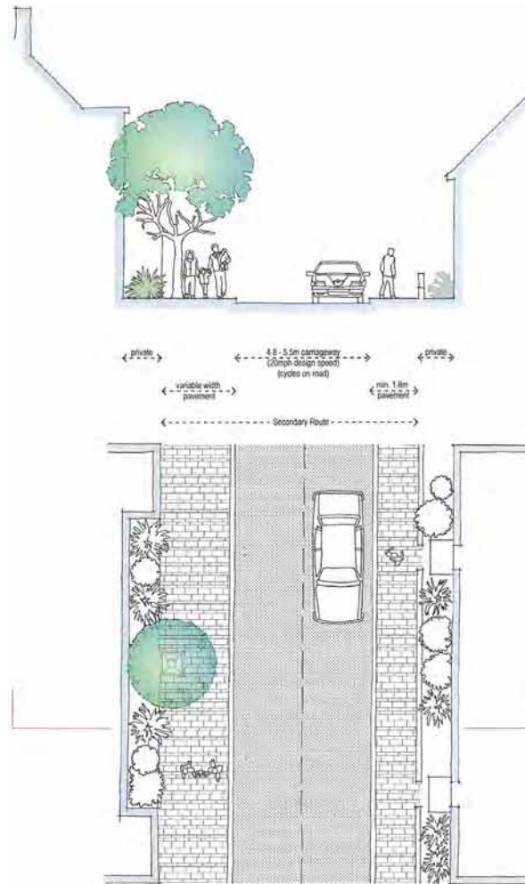
Secondary Route: Proposed typical section/plan
