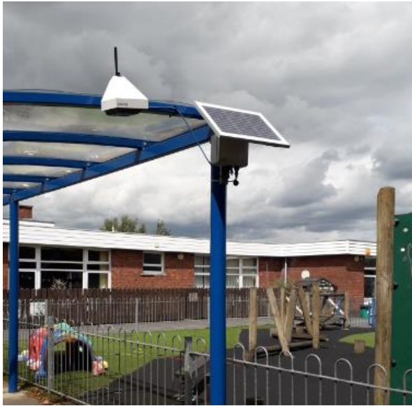
Use of an AQMesh Automatic Analyser to monitor pollution levels at a school.
