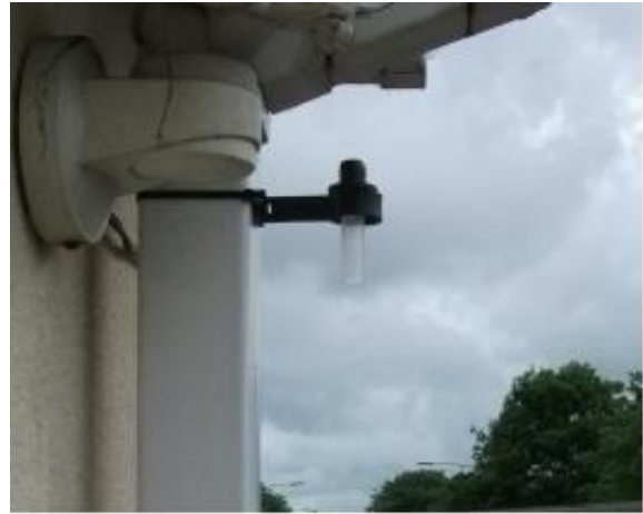
Use of a diffusion tube to monitor roadside NO2 levels from the façade of a property.
